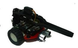
When your TBot is not connected to USB, it will run the last program stored into it's permanent memory when you slide the power switch to "ON".
