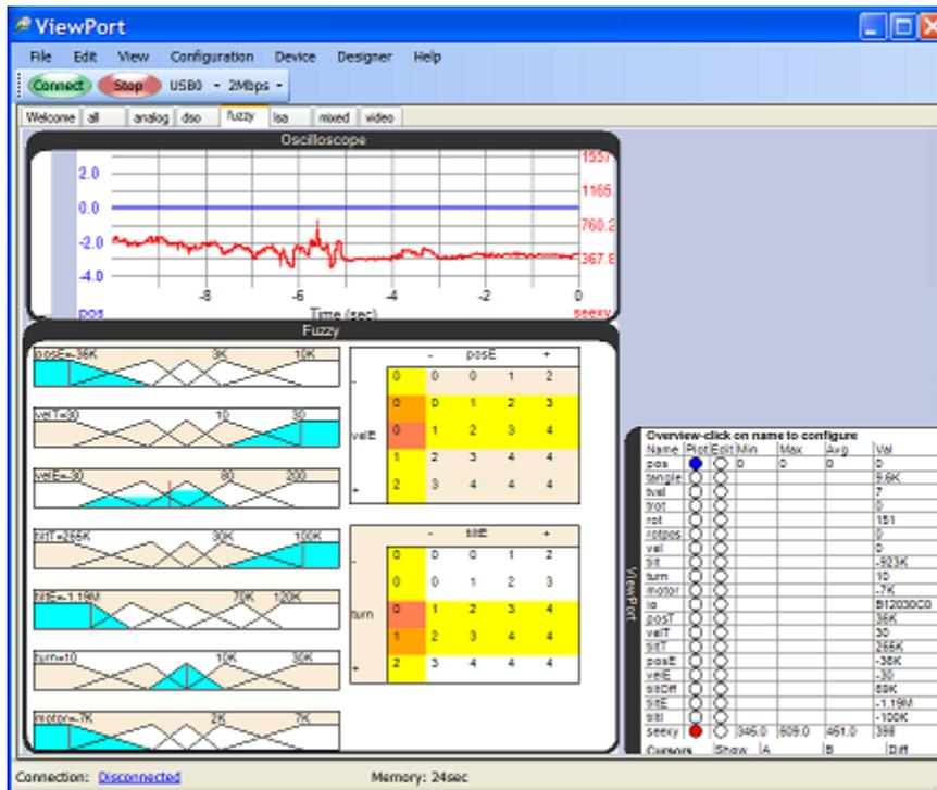
When your program includes a shared fuzzy logic engine, ViewPort enables the fuzzy logic control panel view. This view shows an oscilloscope on top and the overview panel on the right. The Fuzzy panel displays fuzzy maps and fuzzy rules.
