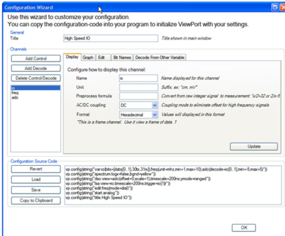
The channels section shows the channels you shared with ViewPort. You can add/delete control and decode channels to this list. The tabs to the right are specific to the selected channel.
