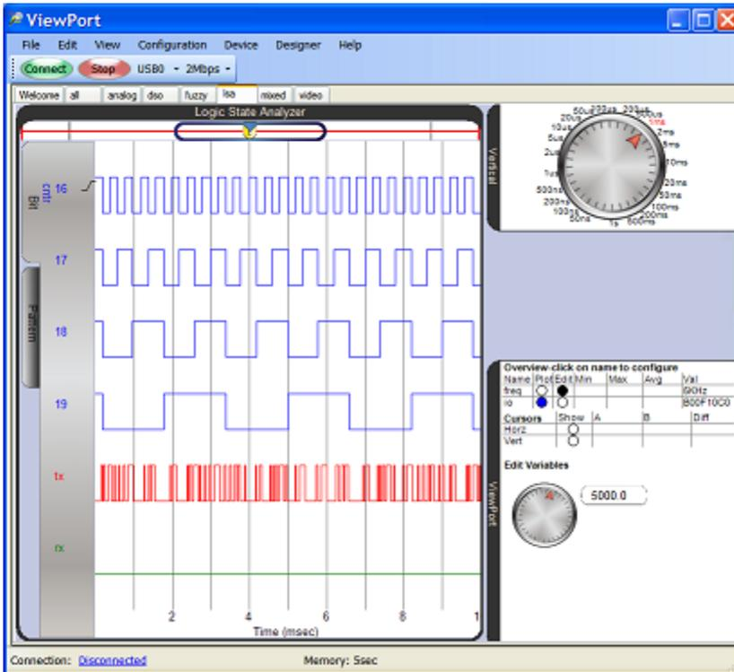
The graph shows the individual bit traces- numbered and labeled on the left. You can change the timescale, time offset, and choose which channel to graph. You can move the traces horizontally by dragging them with the mouse or using the top scrollbar. To change the time resolution use the timescale control. Add and change single bit/edge/pattern triggers by clicking on the bit's label. Use cursors to measure the signal.
